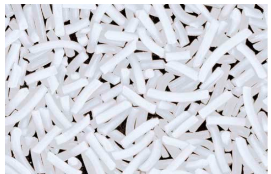
Rod-shaped ceramic grains for high stock removal
